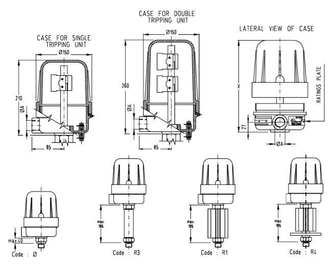
SPACE NEEDED FOR REMOVING THE CASE COVER: X =340 X =440
