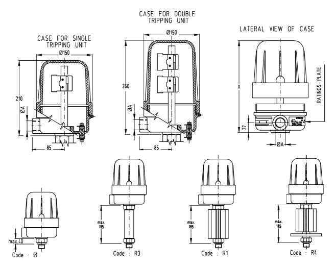
SPACE NEEDED FOR REMOVING THE CASE COVER: X = 340
