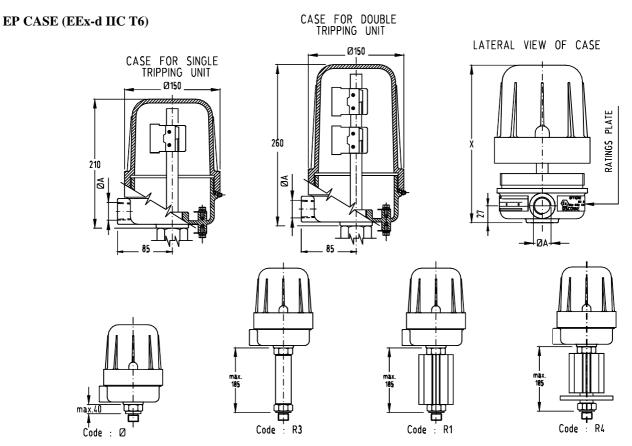
SPACE NEEDED FOR REMOVING THE CASE COVER: X =340 CASE WITH SINGLE TRIPPING UNIT CASE WITH DOUBLE TRIPPING UNIT
