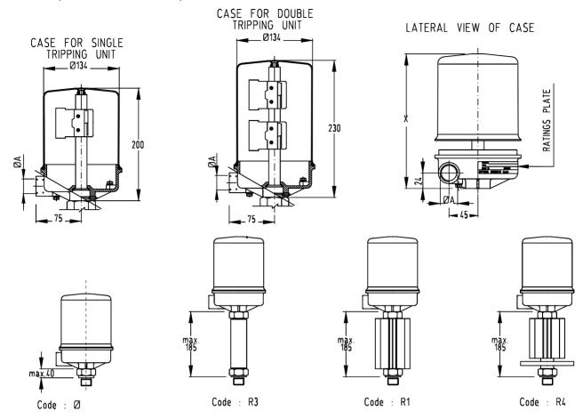
SPACE NEEDED FOR REMOVING THE CASE COVER: X =320 CASE X =400 CASE
