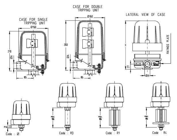
SPACE NEEDED FOR REMOVING THE CASE COVER: X =340 CASE WITH SINGLE TRIPPING UNIT CASE WITH DOUBLE TRIPPING UNIT
