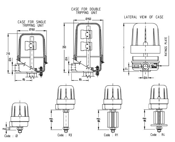
SPACE NEEDED FOR REMOVING THE CASE COVER: X =340 X =440
