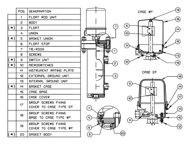
When ordering spare parts, always indicate the instrument's serial number. You can find it on the ratings plate on the case (see Pos.11) and has 5 digits preceded by the letter "F" (e.g.: F45678).
