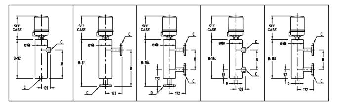
Dimensions to order  $\mathbf{B} = \text{field } \mathbf{C} = \text{connections } \mathbf{D} = \text{draining}$
