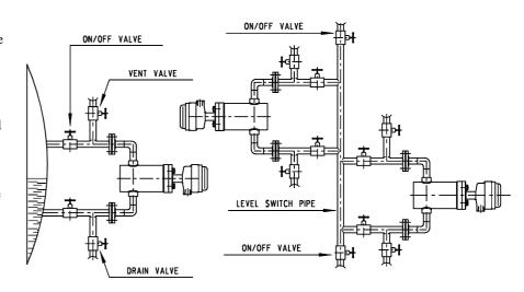
The insertion point on the tank shall be far enough from any obstacle compromising the space necessary for disassembly. Furthermore, the float inside the tank shall be placed in an area free from any liquid turbulence. in case this won't be possible, protections will be provided in order to eliminate the mentioned turbulences.
