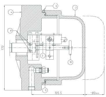
xx necessary space for disassembling
