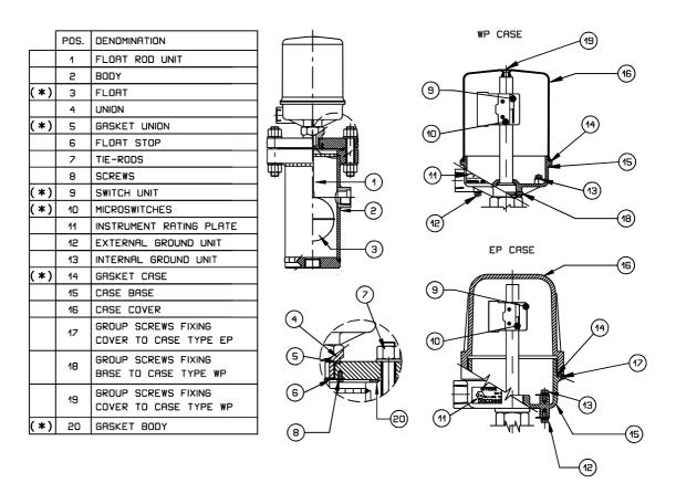
When ordering spare parts, always indicate the instrument's serial number.
