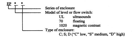
The level or flow switches are made of a flameproof enclosure series EP type C, S, D, containing the magnetic functioning switches or ultrasound switches with their electronic circuit.
