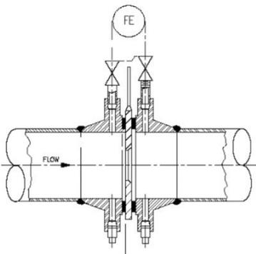
The Meter Run and Flow Meter (FE) are extensions of Orifice Plate flow measurement, where the meters contains the minimum upstream and downstream straight lengths essential for an accurate measurement.
